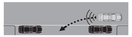
When you determine the vehicle is back far enough or you hear a solid tone from the Reverse Sensing System, bring the vehicle to a complete stop and move the gearshift to D (Drive). The message center will now display PULL FORWARD USE CAUTION followed by a chime.
